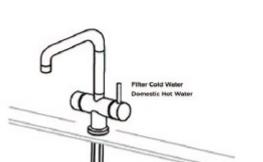
Turn off the incoming cold water supply and disconnect the tap tail from the supply line.
