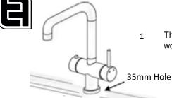
The tap needs a 35mm diameter hole to install into a sink or work top
